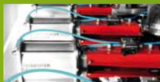
Pneumatically controlled stainless steel valves
